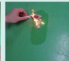
A solvent based epoxy catches fire when it is not diluted with thinner
